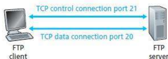
Figure 2.15 ♦ Control and data connections
